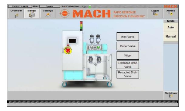
Here, individual control parts of the machine can be manually actuated for testing, maintenance and These include:
